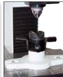
③ Support for anvils to lock the pieces or for quick displacements
