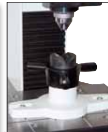
③ Support for anvils to lock the pieces or for quick displacements Code 13330 (optional)
