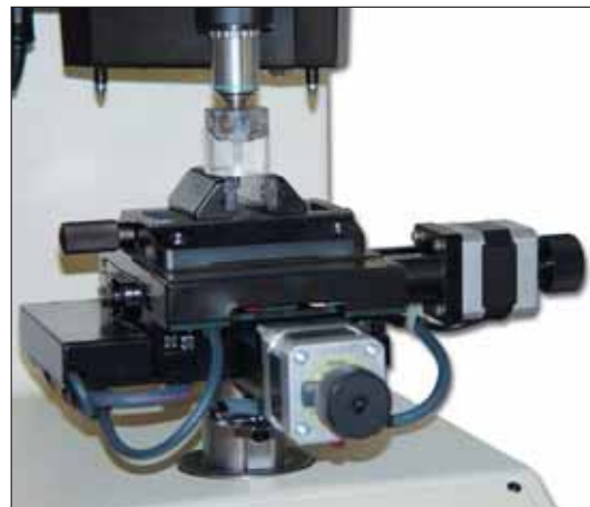
Motorized X-Y table connected with CNC computer for automatic tests ( DM-8 Auto )
