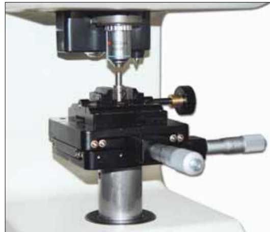
X-Y table 100 x 100 mm 0,01 mm division for easy research of test surface or Zig-Zag tests. AS OPTIONS: 2 Digital micrometers
