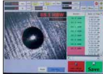
Automatic Brinell / Vickers and Auto Focus
